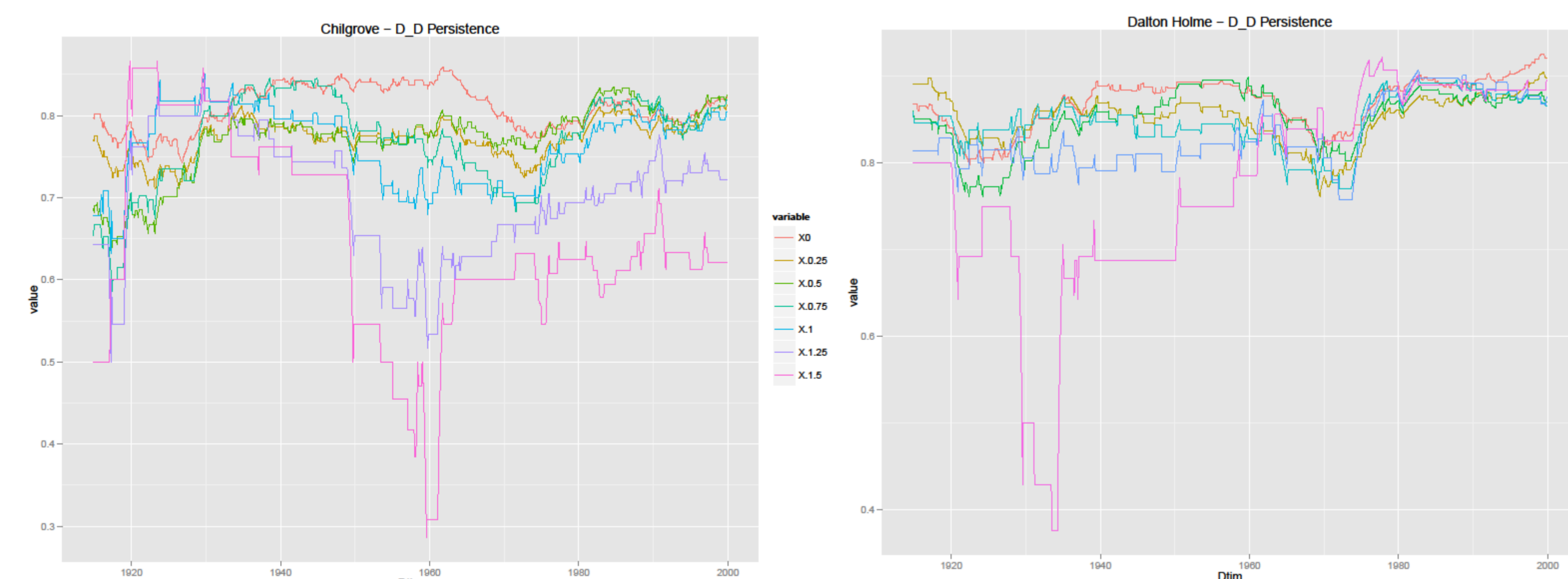
Probability of a 'drought - drought' Markov transition for various SGI thresholds, probabilities derived from a moving 30 year window of observations (data plotted against the centre of the 30 year window).
