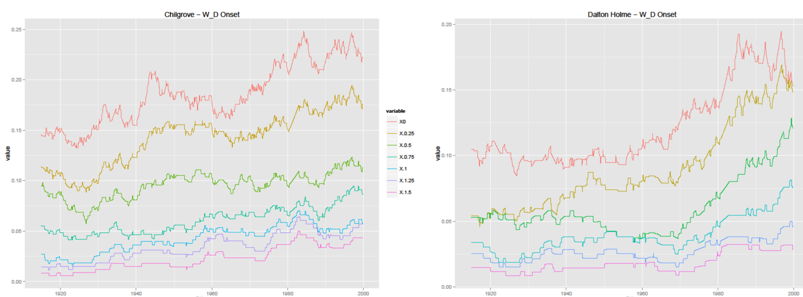
Probability of a 'wet- drought' Markov transition for various SGI thresholds, probabilities derived from a moving 30 year window of observations (data plotted against the centre of the 30 year window).
